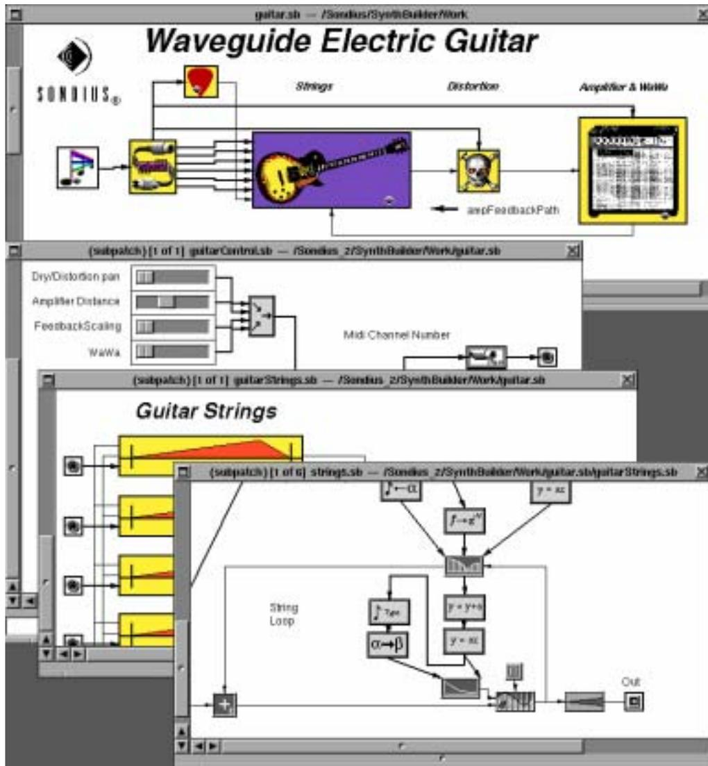
A six string electric guitar model with distortion, feedback and wawa, implemented in SynthBuilder. This model runs on a single 72Mhz Motorola 56002 DSP.
