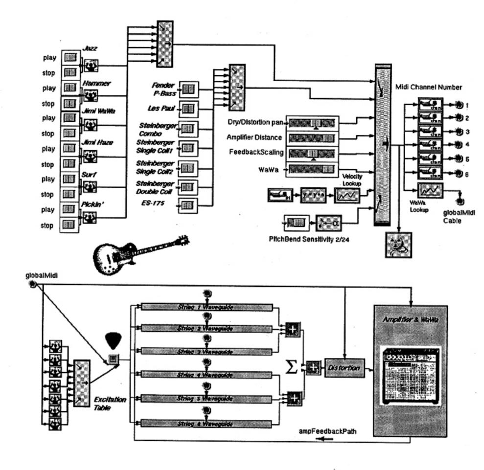
A six string electric guitar model with distortion, feedback and wawa, implemented in SynthBuilder. This model runs on on a single 72Mhz Motorola 56002 DSP.
