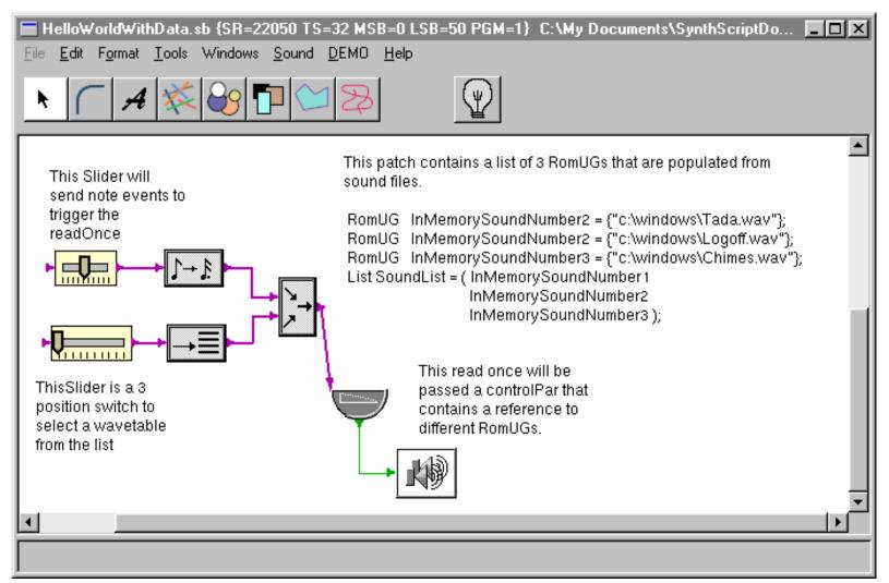
Here is the HelloWorld algorithm modified so that there are 3 RomUGs that are populated from sound files. These 3 RomUGs are collected together into a list, that can be indexed with the indexNF EventFilter. This algorithm uses one slider with a value 0..2 to select which RomUG to pass to the readOnceUG. It uses another slider to trigger the readOnceUG.
